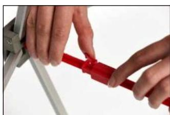
2. Lock the red connectors using the levers on each of them; you can open them by pushing the lever and pulling them apart again
