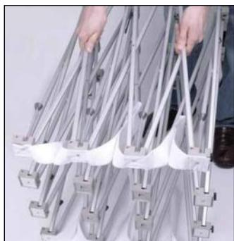
1. Setup the support grid by placing upright on the ground and carefully pulling the grid contraction to full size on the corner sides; one of the sides has small dark bumpers - that's the bottom side of the display
